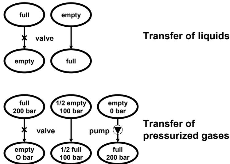
Figure 14 Schematic representation of the transfer of liquids and gases
