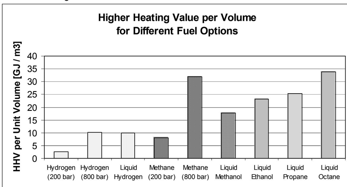
Figure 2 Volumetric HHV energy density of different fuels
