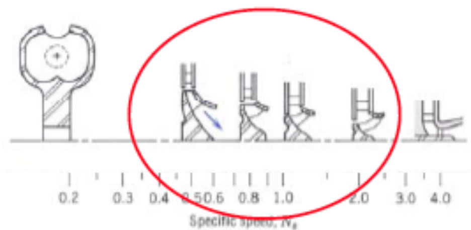
Fig. 11.10 Typical geometric proportions of commercial hydraulic turbines as they vary with dimensionless specific speed [12].
