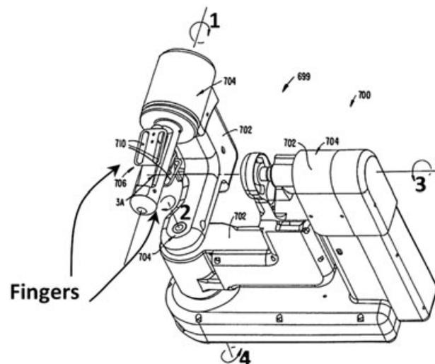
Figure 7. Design details of the da Vinci handle (US Patent No. 6364888B1). The virtual gripper interface, moved by the fingers, allows rotation of the four sensorized joints shown in the figure
