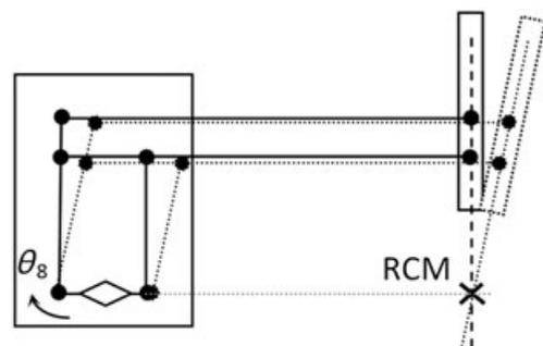
Figure 4. Double parallelogram forming the RCM. Actuation of  $\theta_8$  joint moves the instrument shaft around RCM (terminology adopted from (4))
