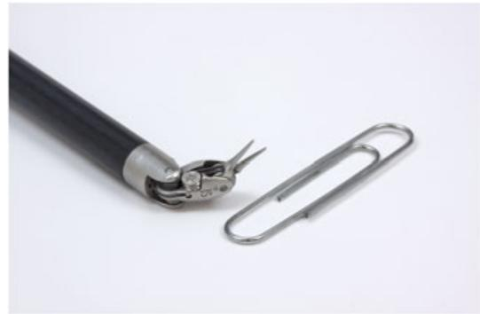
Figure 3. Detail of a microsurgical Endowrist™ instrument (<http://www.intuitive-surgical.com>)
