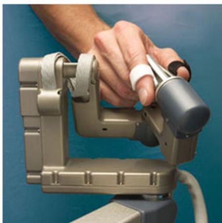
Figure 6. The da Vinci handle used to remotely move the instrument's tip
