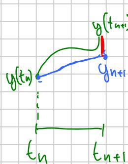
$$\begin{aligned} \tilde{e}_n &= \frac{y(t_{n+1}) - y(t_n)}{h} - \phi(t_n, y(t_n)) \\ &= \frac{1}{h} \left( y(t_{n+1}) - \underbrace{\left[ y(t_n) - h \phi(t_n, y(t_n)) \right]}_{\text{valore esatto}} \right) \end{aligned}$$
