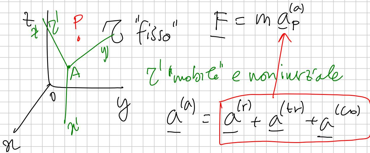
$$\underline{F} = m \left( \underline{\alpha}^{(r)} + \underline{\alpha}^{(tr)} + \underline{\alpha}^{(co)} \right)$$
